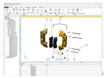
Leverage CAD product structures to dynamically generate parts lists with call outs and maintain associativity with engineering model to automate changes when product design changes occur.
