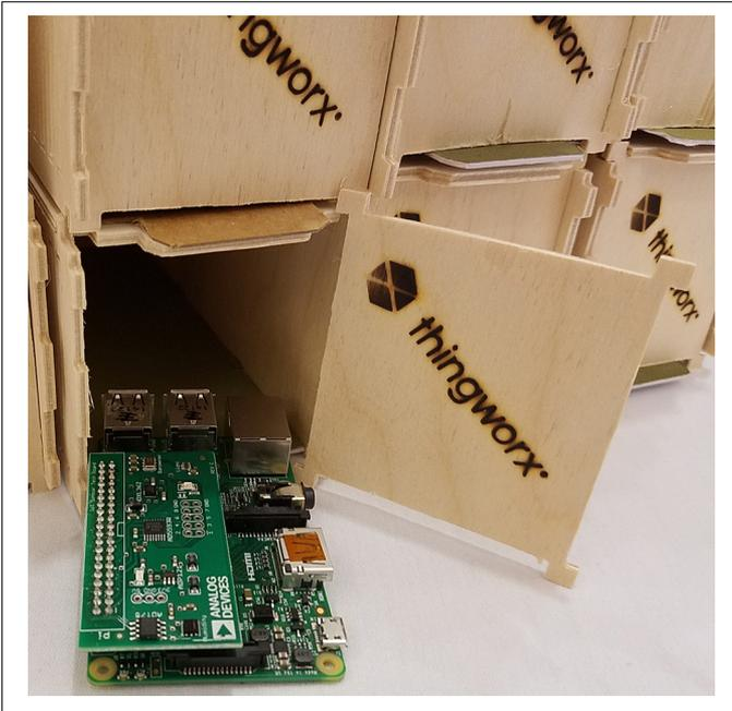
*Figure 1-1. The Raspberry Pi sporting an ADI FAE board*
