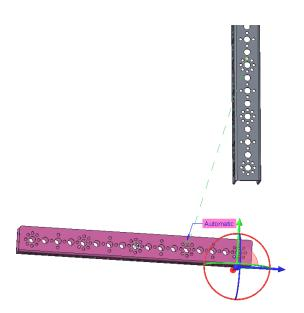
The part appears its natural color after it is placed in the assembly. If you need to change the placement of a part, right-click on the filename in the model tree and select Edit Definition
