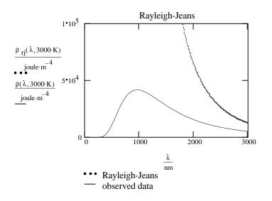
Max Planck assumed that the energy of the oscillators in the blackbody was not continuous, but quantized. He computed the average energy of the oscillators using this assumption. The energy density, dU in the wavelength range  $d\lambda$  is given by the expression:
