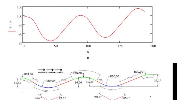
Yes the units are feet. The vehicle (inner Tube) travels from right to left on a wet surface entering the profile at 20 fts.
