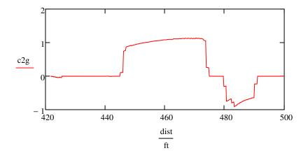
We can see that the centripetal component is sometimes of comparable size to the gravitational component.
