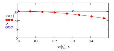
We can see that in free fall the sled would immediately go below the track if the track weren't there; so it's reasonable to assume the sled follows the track profile at the start.
