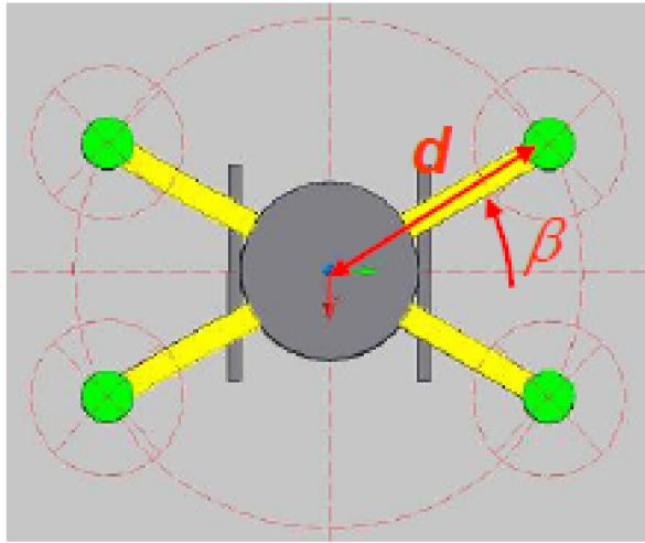
$$\begin{aligned} & \min_{\beta, d} I_{yy} \\ & \text{s.t.: } \begin{aligned} & d \leq d \leq \bar{d} \\ & 0 \leq \beta \leq \frac{\pi}{2} \\ & m_q \leq \bar{m}_q \\ & d \sin \beta \geq \frac{d_r}{2} + f \\ & d \cos \beta \geq \frac{d_r}{2} + f \end{aligned} \end{aligned}$$
