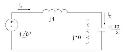
The delta to wye conversion reduces the balanced capacitance by a factor of 3. Finding the current la:
