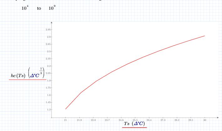
Note that the above heat transfer coefficients do not include the effect of radiation. If a combined heat transfer coefficient is to be calculated, the radiative heat transfer coefficient hr must also be calculated. Usually, hr is calculated as follows:
