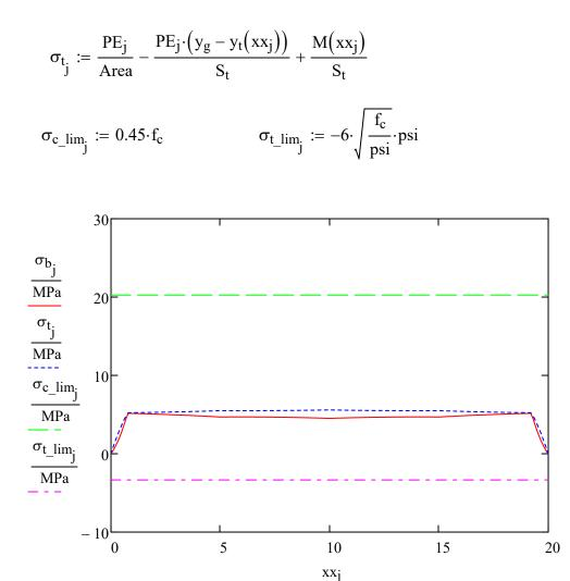
Note how for the example the full service level condition is very favourable, since the full beam remains compressed around the average 5 MPa level. However the beam has to have too much depth for our taste, due to uncommon loading.
