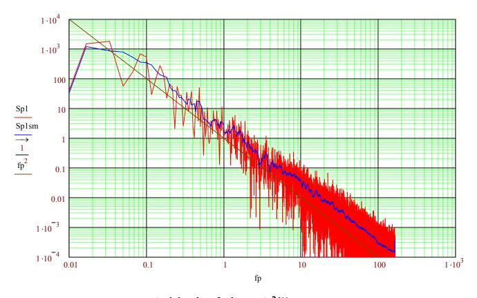
power spectral density of p in counts  $^2/Hz$  red: PSD, blue: smoothed PSD, brown:  $1/f^2$
