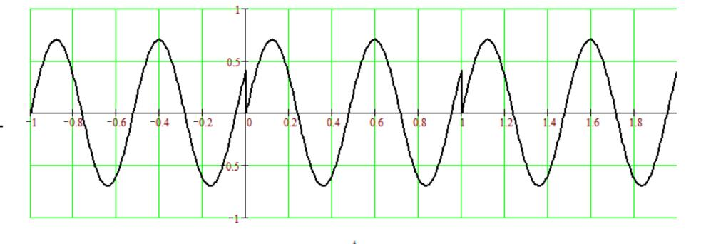
Effective periodic waveform for DFT of sinusoid with f = 2.1, and sampling period of T = 1. Repeating waveform from the interval  $\{0,1\}$  does not result in a pure sinusoid, resulting in multiple Fourier series coefficients. The DFT reconstructs to the Nyquist band-limited version of the sampled input.
