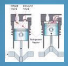
Operation depends on camshaft speed, physical dimensions of the pistons, fluid intake conditions and Gas Laws
