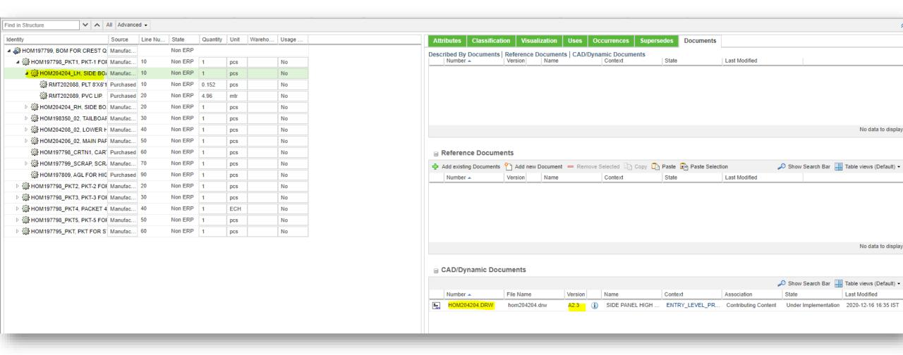
BOM structure with multilevel WT part structure WT parts are linked to CAD drawing. Here highlighted WT part is linked with CAD drawing.
