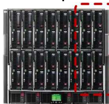
Current Production SAP HP Blade System c7000 Enclosure 16 single blade units 6 single units available
