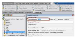
When the assembly is checked in to Windchill, the Component Name appears for each Windchill CAD document
