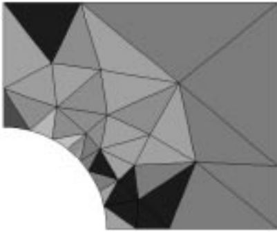
Figure 7 Von Mises stress in 1/4 model of thin plate under tension using first order elements
