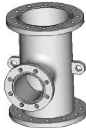
Figure 13 A hypothetical 3D solid model of a piping junction
