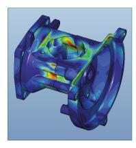
Pro/ENGINEER Mechanica enables validation of designs, such as this model of a bolted housing, and reduces the number of physical prototypes needed.
