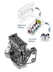
Pro/ENGINEER Advanced Assembly Extension offers capabilities, such as skeleton models, to support top-down design.
