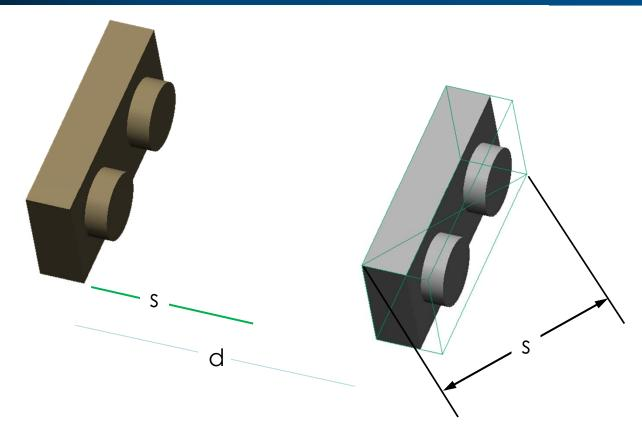
If  $d \le t^*s$  then the constraint becomes coincident. Otherwise it becomes a distance constraint. <u>UNITS ARE NOT CONVERTED!!!</u>
