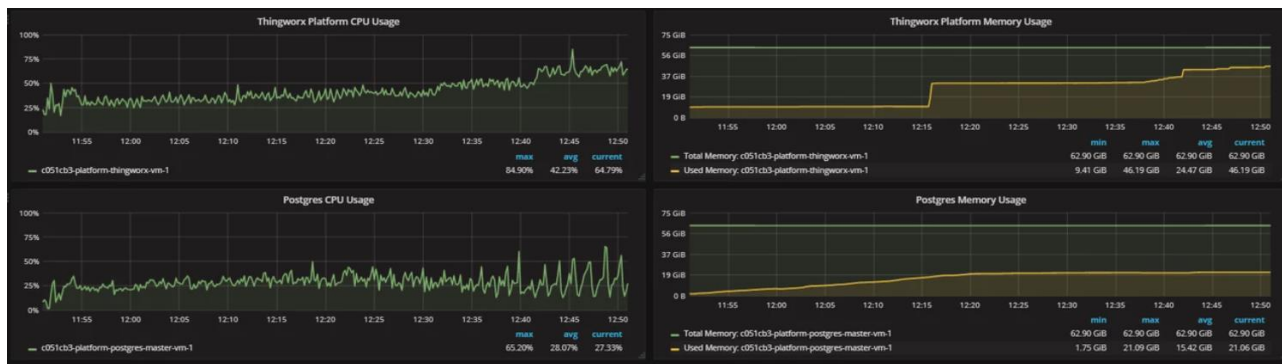
FIGURE 4 – THE THINGWORX CPU IS ABOUT THE SAME HERE AS IN THE INFLUXDB CONFIGURATION BELOW BUT LOOK AT HOW MUCH MORE MEMORY BOTH THE PLATFORM AND THE POSTGRES DATABASE NEED ALLOCATED TO THEM IN THIS CONFIGURATION (64 GB A PIECE).
