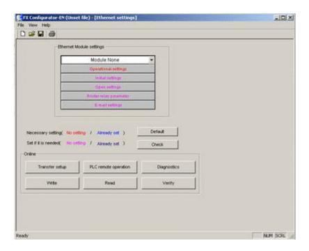
3. Next, specify the FX3U-ENET block's minimum required configuration information. Select a module from the first drop-down list and then click **Operational Settings**.
