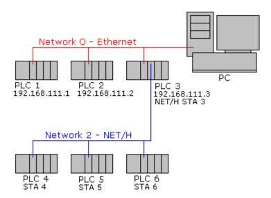
If PLC 1, PLC 2 and PLC 3 have QJ/1E71-100 Ethernet modules configured with IPs 192.168.111.1, 192.168.111.2 and 192.168.111.3 respectively. In addition to the Ethernet module, PLC 3 also has a QJ/1BR11 NET/H module configured as station 3. Assume that PLC 4, PLC 5 and PLC 6 have NET/H modules configured as stations 4, 5 and 6 respectively.
