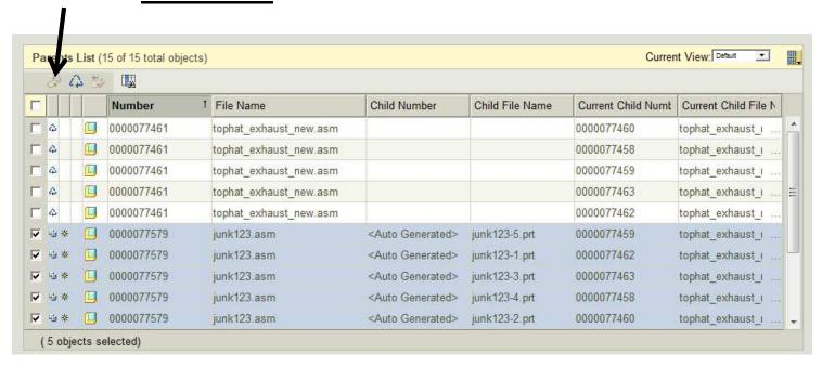
CHECK AS SHOWN. THEN SELECT ICON NOTED WITH ARROW \*. PARTS WILL BE SWAPPED IN JUNK123.ASM WITH JUNK123-1, ETC.
