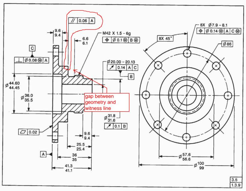
FIG. 3-25 FEATURE CONTROL FRAME PLACEMENT
