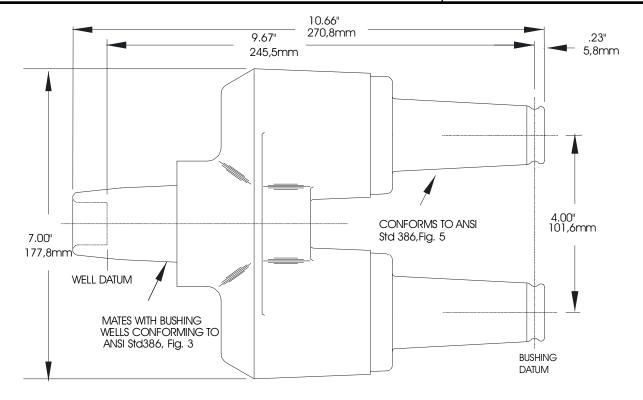
The Elastimold 1602A3R feed-thru bushing insert is fully rated with a 15kV class, 200 Amp load break bushing interface. The feed-thru bushing insert fits a standard ANSI bushing well interface and provides the capability of creating a tap position in an existing apparatus installation and transforming a radial-feed transformer into a loop-feed unit.
