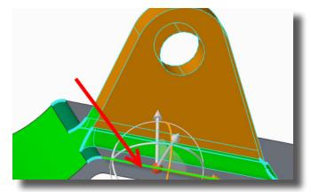
69. **LMB** select and drag the orange arrow right until a value of **0.28**. (You can directly enter the value by clicking on the dimension)
