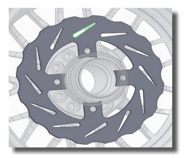
29. Zoom in on the <u>upper</u> mounting tab of the rotor part. **LMB** select the cylindrical surface of the hole as shown
