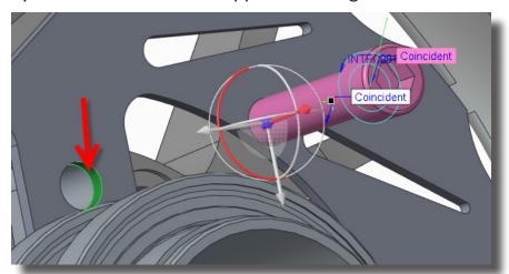
39. LMB select the top surface of the upper mounting tab on the rotor part as shown
