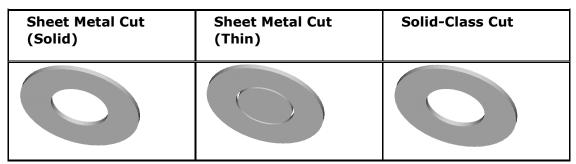
Because sheet metal cuts are surface cuts, you cannot make a cut to partially remove wall thickness. For example, you can not cut a 1cm deep hole in a 10cm thick wall. This may make the Blind depth command somewhat difficult to understand. The Blind depth command applies to cutting on bends. You can sketch the cut to the edge of the bend and project it a blind depth down the bent wall, saving you the time of unbending the wall, making the cut, and bending back the wall.
