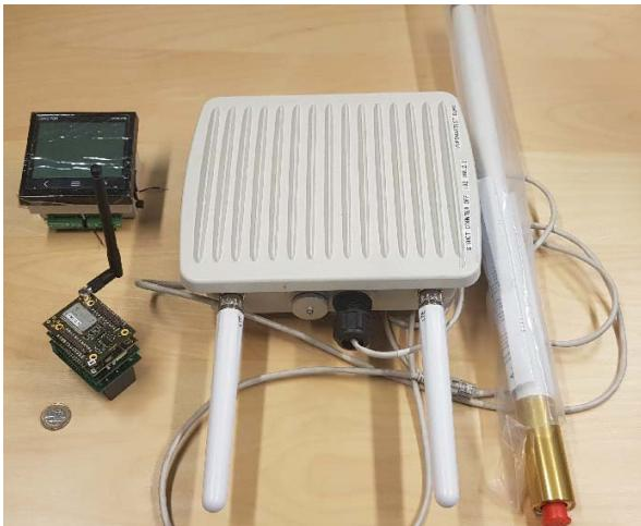
Fig. 3. Used hardware: a sensor node, power meter and LoRaWAN gateway with 868 MHz antenna (in plastic bag)
