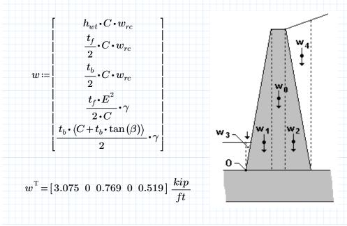
Distances from the area centroids of segments to the face of the wall at top of footing:
