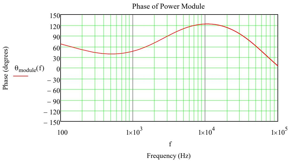
Want the total loop to cross at a decade or more before the module's crossover. To do this, determine what the gain of the module is at the desired system crossover frequency, determine the contribution from the open loop load share components, then select the error amplifier components to add the desired attenuation
