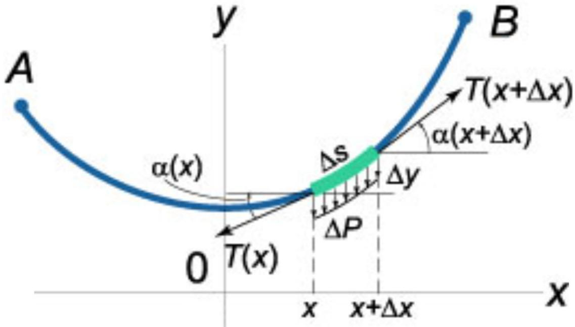
$$\Delta P = \rho \cdot g \cdot A \cdot \Delta s \quad A - \text{chain cross section}$$
