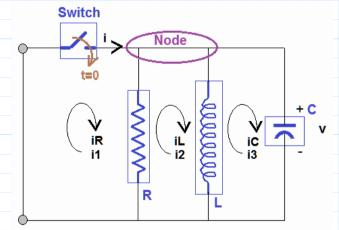
Parallel RLC circuit, here we want to solve for voltage because the voltage is the same across the parallel branches. At the Node the voltage would be the same where all three passive elements R L and C are connected.
