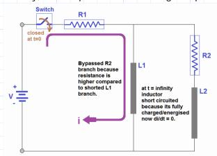
When switch is closed, inductor L1 and L2 get fully charged-energised, it becomes a short circuit.
