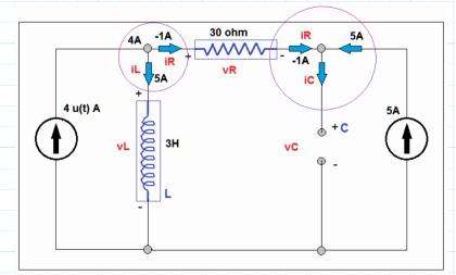
Discussion: What remains is the capacitor current and voltage. We had iC(0-) = 0. But now there is an abrupt change in current, since left side source 4A has come ON. It will cause voltages to change. We cannot expect a vC change because of current change. We see dvC/dt exist for t=0+, when 4u(t)A came on at t=0.
