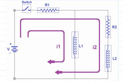
Form 2 loop equations to solve the circuit. We set two currents i1 and i2 then apply Kirchoff Voltage.
