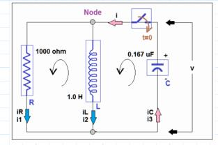
RLC parallel circuit with node. You may sketch a better looking circuit. Take into consideration its a source free circuit and capacitor is the source of voltage and current.
