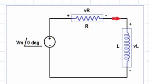
Current I is obtained as a function of s, by dividing voltage by impedance.
