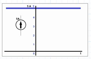
At time t=0-, the 4u(t) source was not supplying current. But the current source on the RHS supplied current of 5A for time t=0-. At t=0 and t=0+ both the LHS and RHS are supplying current i.e. 4u(t) A and 5 A.
