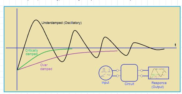
Figure above shows, dependent on input-source, dependent on circuit, the output response are three cases; under, critical, and over damped.
