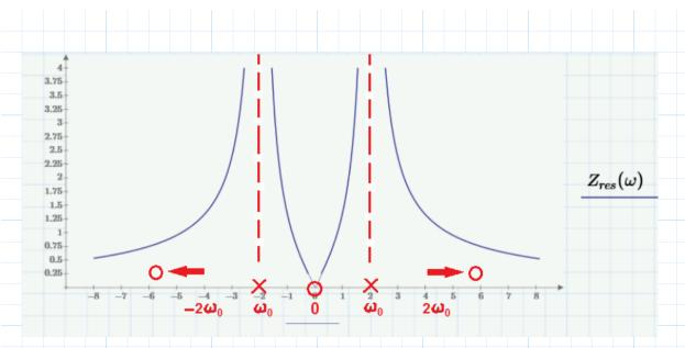
Location for critical frequencies are marked on the w-axis using small circles for zeros and crosses for poles. Poles or zeros at infinity frequencies should be indicated by an arrow near the axis, as shown figure above.
