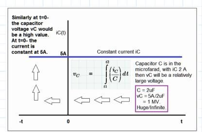
Capacitor voltage an unrealistic high value or infinite value at t=0-
