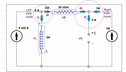
Left side node, we have 0 current entering the node from 4u(t). Shown on figure.
