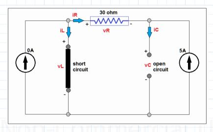
The three voltages and currents can be found by resistive circuit analysis.
