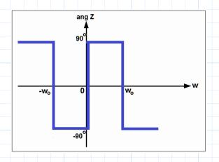
L and C get their current at the same time, when one is at 90 deg +ve because its lagging (L), the other is at -90 deg -ve because its leading (C).
