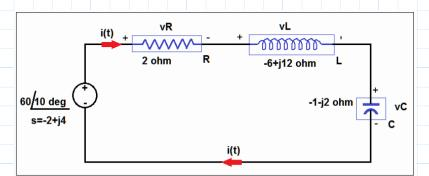
Frequency domain equivalent of resistive circuit.
