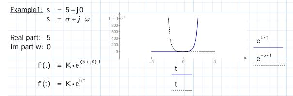
This is all the information we have. K? Well if K is real its a real physical system. In electrical it need not be real, it can be imaginary. With exponent +5 the curve will rise upward (blue) and -5 it drops to 0 (black).
