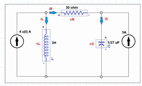
Illustrate the procedure and find a*lll* these values by the careful analysis of the circuit in the figure above. To simplify the analysis numerically an unrealistically large capacitor is used.
