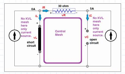
From observation there is only one mesh, as opposed to three. The left side and right side mesh do not have voltage because they are only current source branches.
