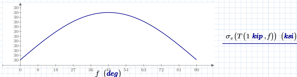
Figure 2: Von Mises stress VS reference plane angle
