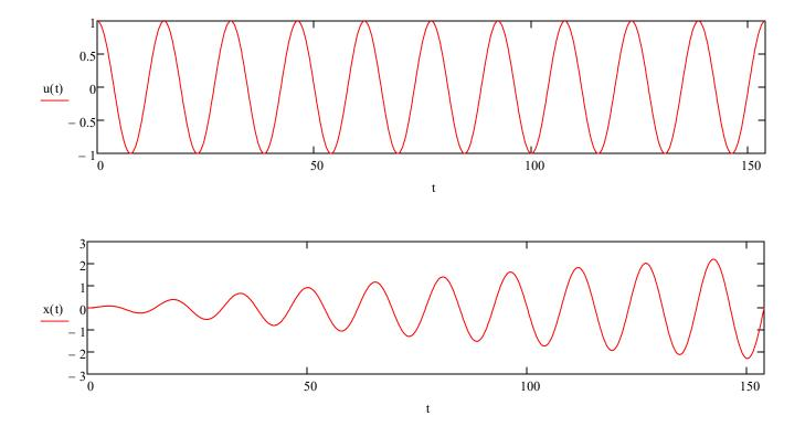
Using odesolve makes calculating the amplification factor more difficult. You have to dump the odesolve 'function' output into matrices, so that the max displacement can be calculated.
