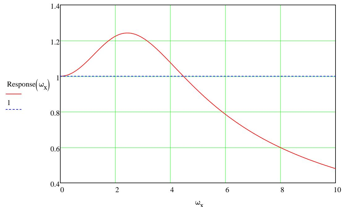
The figure shows the response of the compensator. The peak corresponds to undamped natural frequency for the system. Peak is high above 1 and system should never be used for these frequencies. Dotted lines shows where the response becomes 1 for frequencies below this point
