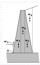
Distance from the area centroids of segments to the face of the wall at the top of footing:
