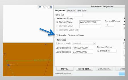
Notice there is a check mark next to Rounded Dimension Value on the vertical dimension and missing from the horizontal dimension
